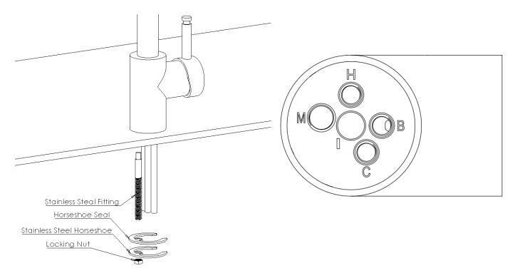
Feed the tails through the countertop and screw fitting into thread 'M'. Slide on horseshoe fittings as shown and tigthen with the locking nut.
