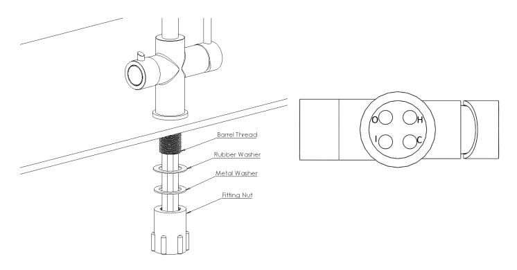
Feed the tails through the barrel thread and hand tighten into the tap. Fit the tap in the desired location using the black plastic fitting nut.
