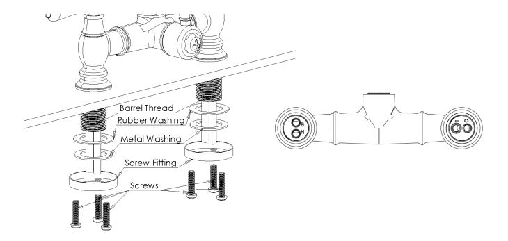
Feed the tails through the barrel thread and hand tighten into the tap. Fit the tap in the desired location using the locking nut and accompanying screws.
