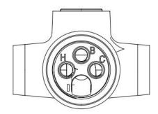
Feed the tails throught the barrel thread and hand tighten into the tap. Fit the tap in the desired location using the locking nut and accompanying screws.
